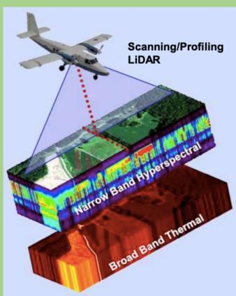
Figure 3. Overview of the G-LiHT imager including a look at how the Lidar, hyperspectral and thermal imager all work together. (University of Alaska Fairbanks Hyperspectral Imaging laboratory, 2013).
